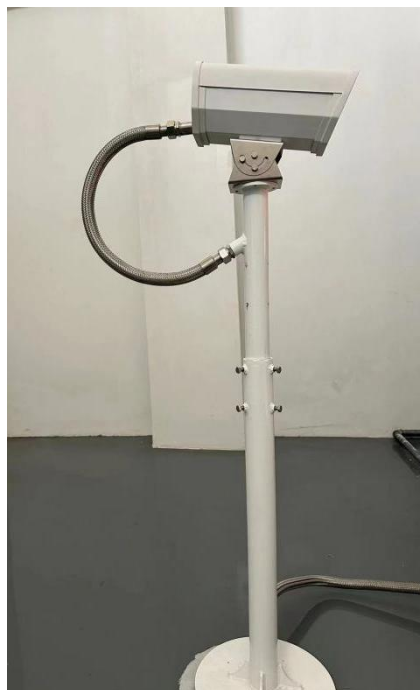
Figure 1 Application of HIRDA-LT high protection infrared thermal imaging detection and analysis system
